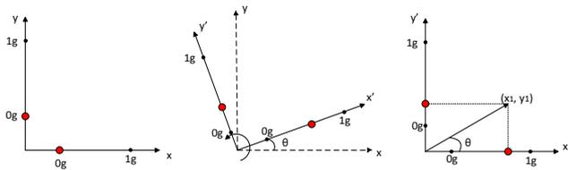
Fig. 3. Calculation of angular position using accelerometer
