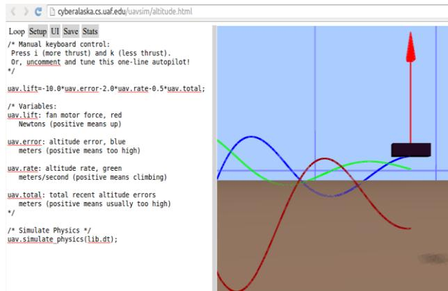
Fig. 7. AERO-Beam web simulator interface. The “error”, “rate”, and “total” terms correspond to the proportional, derivative, and integral terms of a PID controller.
