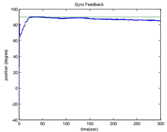
Fig. 5. Control results with gyroscope feedback alone
