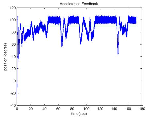
Fig. 4. Example for calculation of angular position using accelerometer
