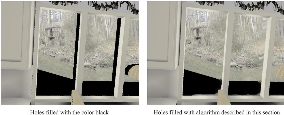
**Figure 3.10:** *Good-quality hole filling is important. On the left is a frame in which holes are filled with the color black. On the right is the same frame in which the holes are filled with the algorithm described in this section. Later in this section, Figure 3.20 provides a more detailed comparison of hole-filling algorithms.*
