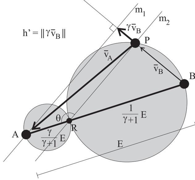
**Figure 3.29:** Transition between hole-size case #1 and case #2. The transition occurs when point  $P$  lies at the edge of the grey circles. The interior of the circles represents the region in which case #2 is applicable.
