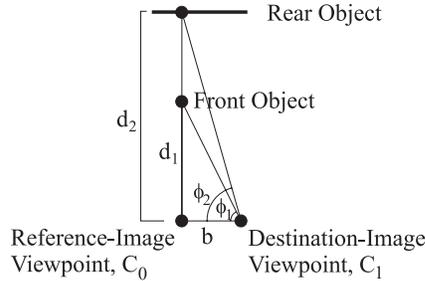
**Figure 3.3:** Dimensions for approximate calculation of visibility-hole size.
