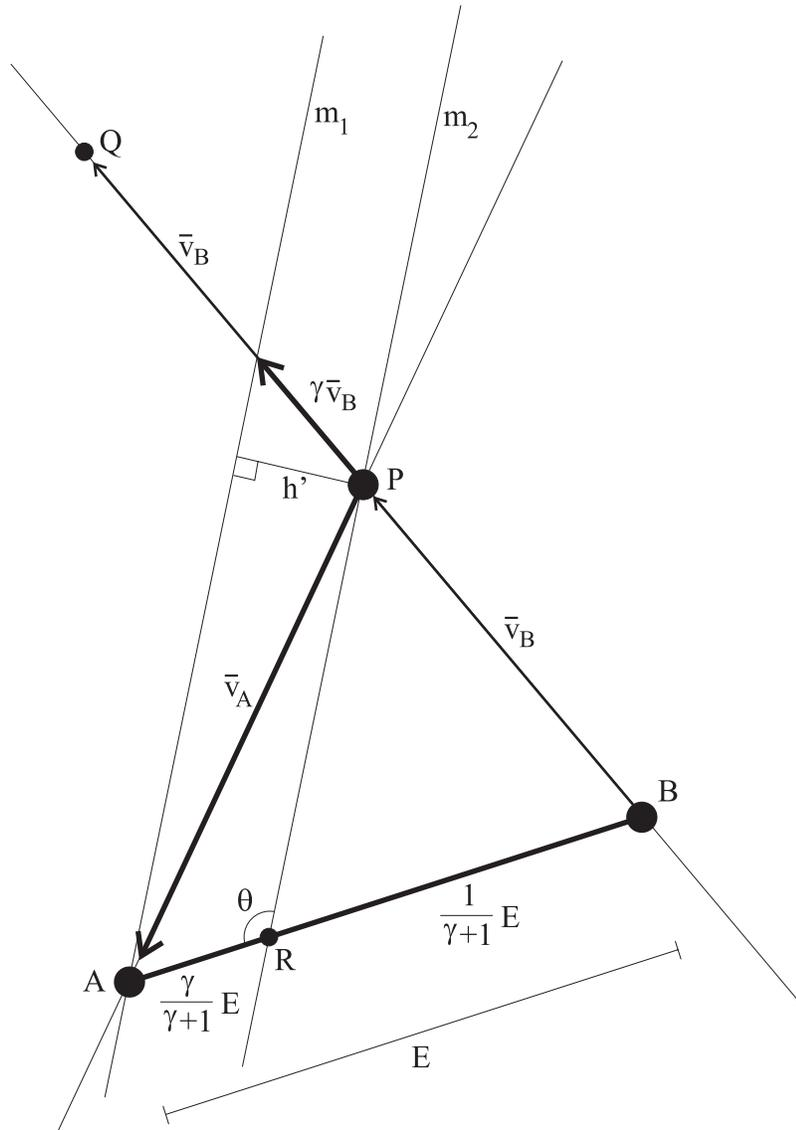
**Figure 3.28:** Geometric argument for bound on hole-size  $h$ , under case #1.
