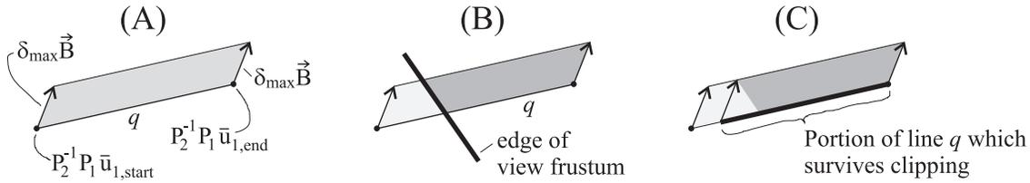
**Figure 5.12:** Clipping for the 3D warp. (a) Possible locations of warped pixels from a reference-image scan line. These locations form a parallelogram in the displayed image’s projective coordinate system. (b) The parallelogram is clipped against the displayed image’s view frustum. (c) The clipped vertices are then used to determine the extent of the reference image line which must be warped.
