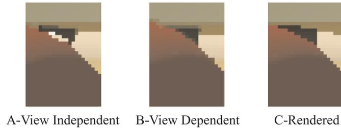
**Figure 4.8:** *View-independent vs. view-dependent surface segmentation. (a) Shows the results from my previous, view-independent, technique. A gap incorrectly opens between the red foreground object and the brown mid-ground object, allowing the yellow/tan background to show through. (b) Shows the results from my view-dependent technique. (c) Shows the results from conventional rendering.*
