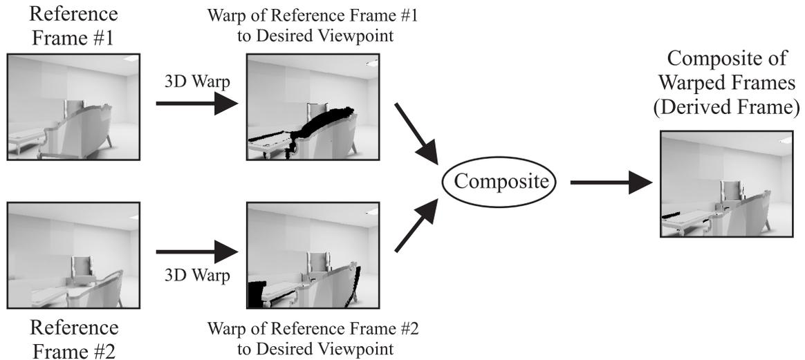
**Figure 3.4:** A single warped frame will lack information about areas occluded in its reference frame. Multiple reference frames can be composited to produce a more complete displayed frame. (For illustration purposes, the inter-viewpoint distances are much larger than normal, resulting in larger-than-normal-sized visibility holes).
