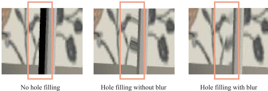
**Figure 3.17:** *Hole filling with and without blurring. The left image shows the unfilled hole. The hole is the black area inside the pink box. The middle image shows the results of my epipolar-geometry-based hole-filling algorithm, but without blurring. The right image shows the results of my algorithm with blurring. The blurring reduces the perceivability of the hole.*
