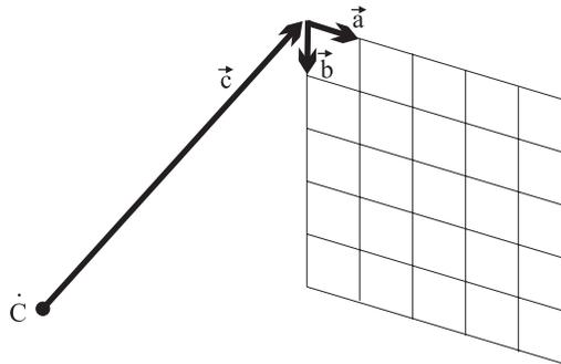
**Figure 1.5:** Alternate, resolution-dependent, camera model for planar projections.
