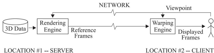
**Figure 6.1:** *Remote display system.*
