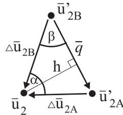
**Figure 3.27:** Angles and lengths for hole-size computation.
