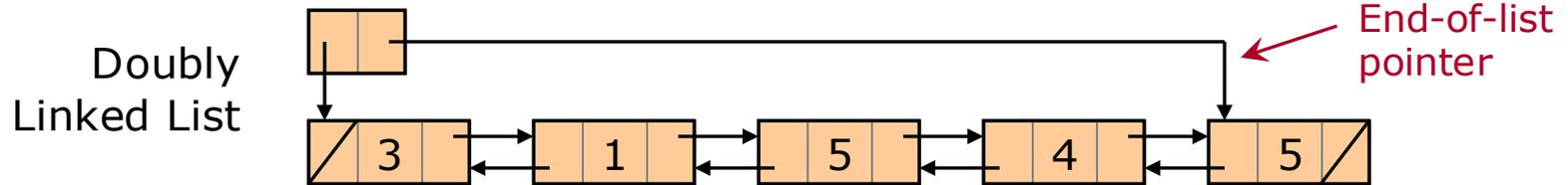
A Doubly Linked List typically has an end-of-list pointer. This can be efficiently maintained, resulting in constant-time insert and remove at the end of the list.
