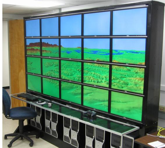
Figure 4: The UAF CS Bioinformatics powerwall, running the *soar* terrain renderer used for benchmarking.
