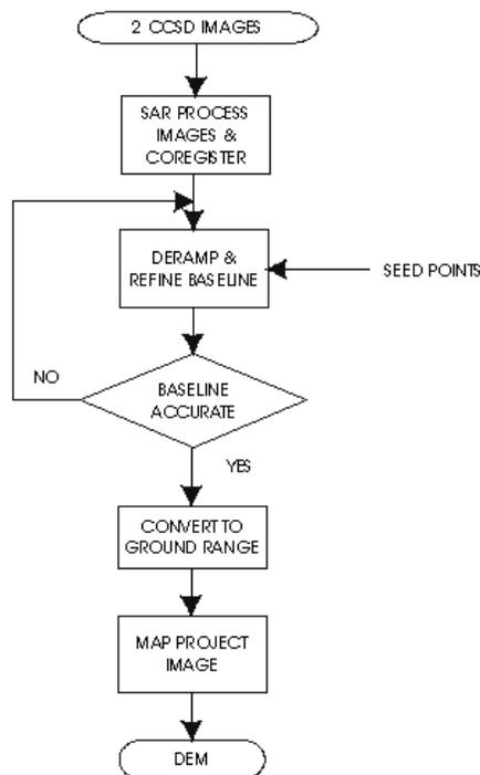
Figure 2: Software Flow Diagram
