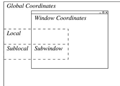
Figure 3: Coordinate systems used inside MPIglut.
