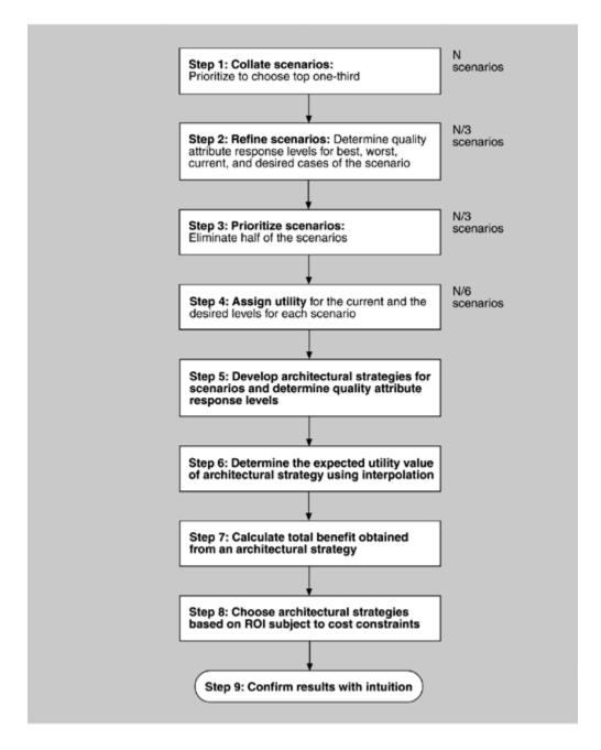
Figure 11: Process flow diagram for the CBAM
