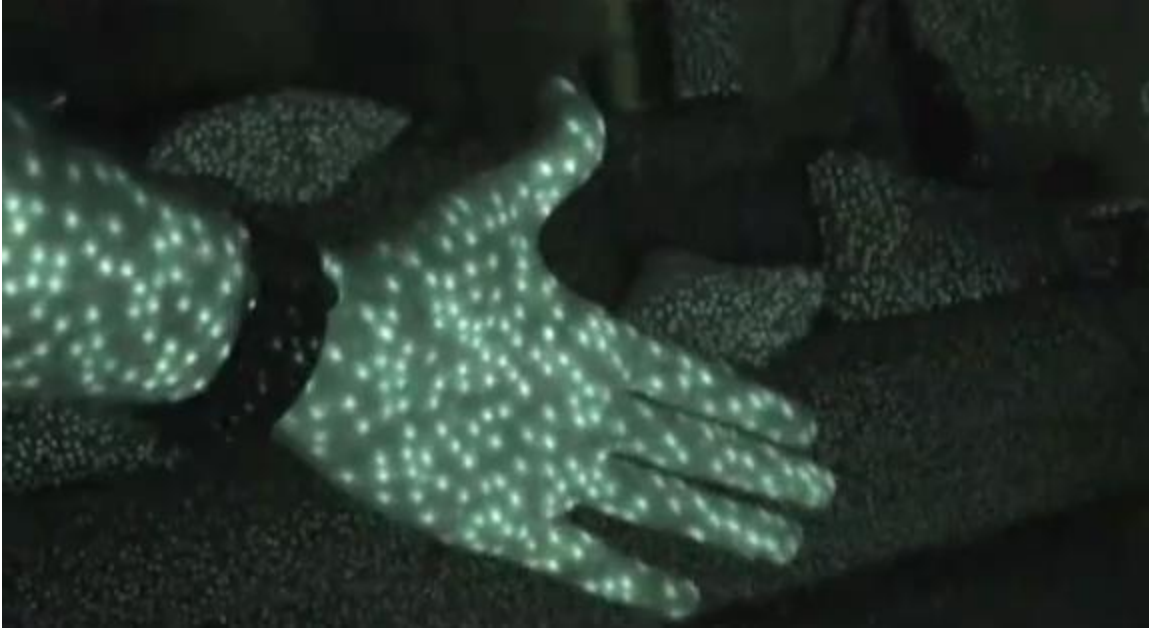
FIGURE 5: IR DOT PATTERN EMITTED BY THE KINECT
