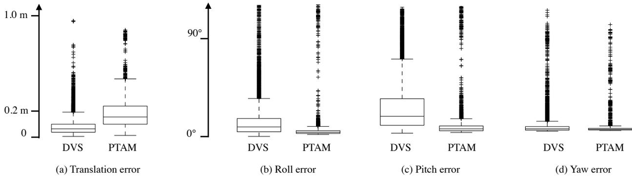
Fig. 8. Distributions of the errors of DVS/PTAM in reference to the OptiTrack measurements. The data is synthesized in Table III.
