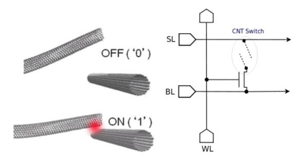
From reading a few papers, this process is quite difficult to perfect, and the fastest I saw for write low was 50ns and write high 500ns. The write speed is a bit slow when compared with DRAM speeds. The theoretical intrinsic set/reset speeds of NRAM is <1ns but this does not have any working prototypes.
