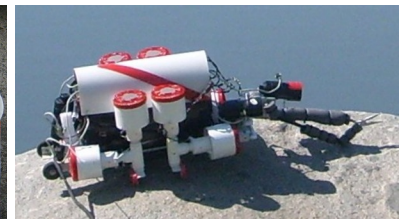
2008 UAF underwater robots PIC 16F882 microcontroller ST Micro VNH3SP30 H-Bridges Competed at MATE ROV finals in San Diego, California "Inspiration for Future Engineers" Award
