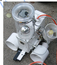
2008 UAF underwater robots PIC 16F882 microcontroller ST Micro VNH3SP30 H-Bridges Competed at MATE ROV finals in San Diego, California "Inspiration for Future Engineers" Award
