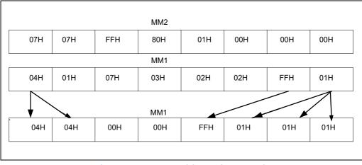
Figure 4-6. PSHUB with 64-Bit Operands
