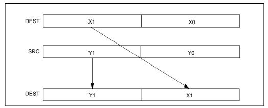
Figure 4-16. UNPCKHPD Instruction High Unpack and Interleave Operation
