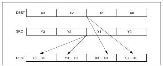
Figure 4-15. SHUFPS Shuffle Operation
