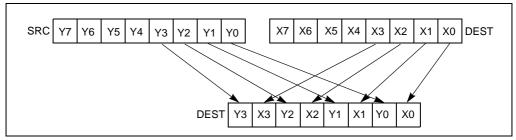
Figure 4-12. PUNPCKLBW Instruction Operation Using 64-bit Operands
