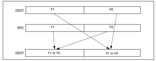
Figure 4-14. SHUFPD Shuffle Operation
