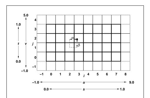
Figure 3.10. A texture image and the coordinates used to access it. This is a twodimensional texture with n = 3 and m = 2. A one-dimensional texture would consist of a single horizontal strip.  $\alpha$  and  $\beta$ , values used in blending adjacent texels to obtain a texture value, are also shown.
