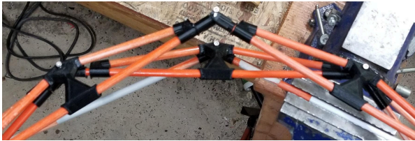
Scaled up origami design, composite rods with defined motion along 3D printed joints.
