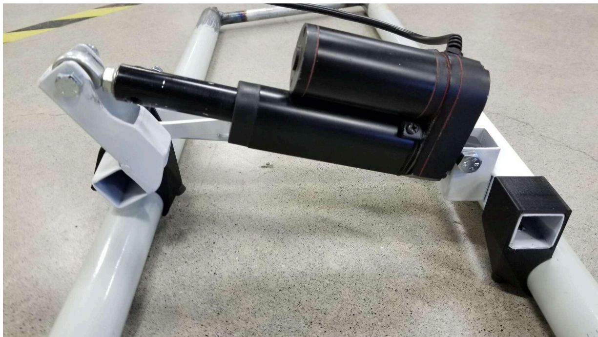
Welded tube truss, gripped by prototype robot end effector, which leveres the rotating left gripper outward to grip the parallel truss tubes.
