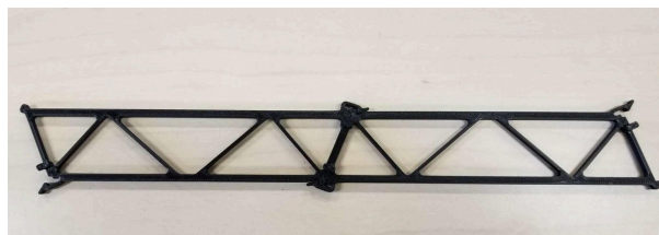
Rotating one module 180 degrees results in a straight segment, for flat roofs, floors, or walls; or towers.
