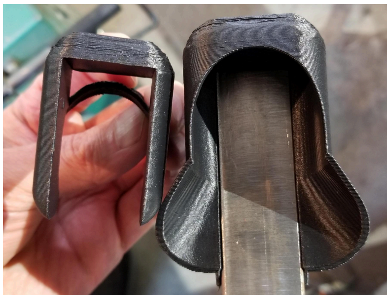
Latest hybrid truss design using small 3D printed capture funnels for easy robotic alignment, while retaining the strength of metal-to-metal contact along the endplates. This iteration also includes basalt fiber diagonal tension rods, and a small spring-loaded capture pin for full push-connect operation.
