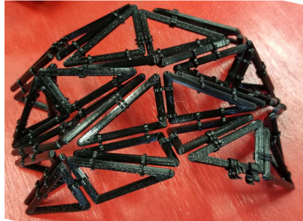
Origami packaging with discrete rigid truss segments. To support a heavy regolith cover, the tubes and connections need to be thick, which complicates origami-style deployment.
