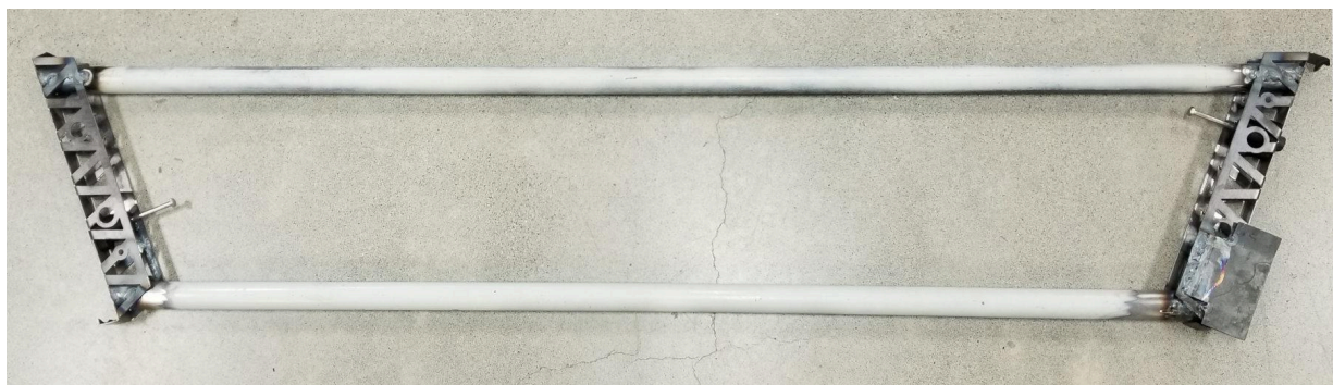
Upgraded plasma-cut endplate truss included an aligning feature, and locking pins.
