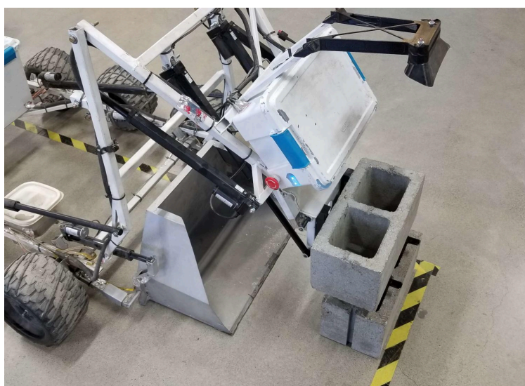
Full scale teleoperated test of our multipurpose robot stacking cinderblocks (17kg) with forklift-style forks.
