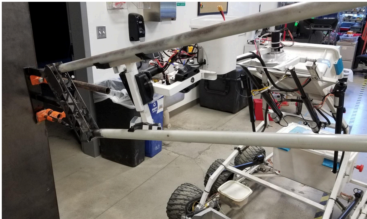
Plasma-cut endplate flat L-truss, demonstrating docking attempts (unsuccessful) with robot arm.
