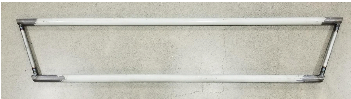
Our CDR design used welded tubes , which was strong but difficult to manufacture.
