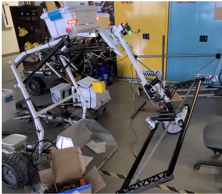
Excavator lifting a truss segment in the lab.
