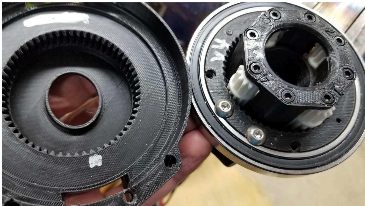
Open gearbox showing the output ring gear and planet carrier, which is numbered for the corresponding planets (which are each individually timed to the ring gears).
