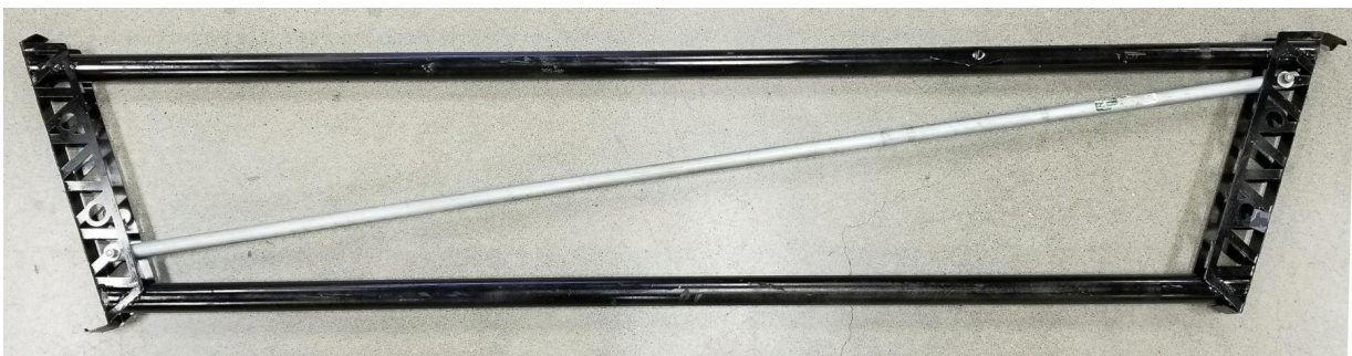
Plasma-cut endplates simplified manufacturing, but were still difficult to robotically push connect.
