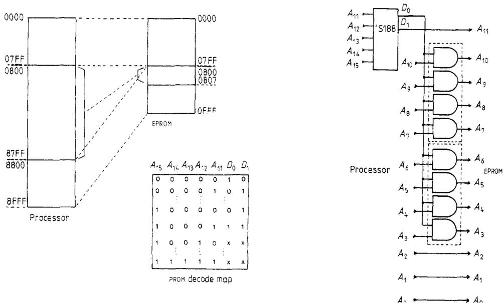
**Figure 4.** PROM decode and mapping.
