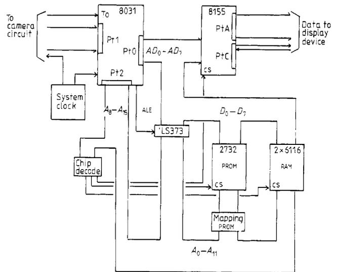
Figure 2. The 8031 microprocessor control system.
