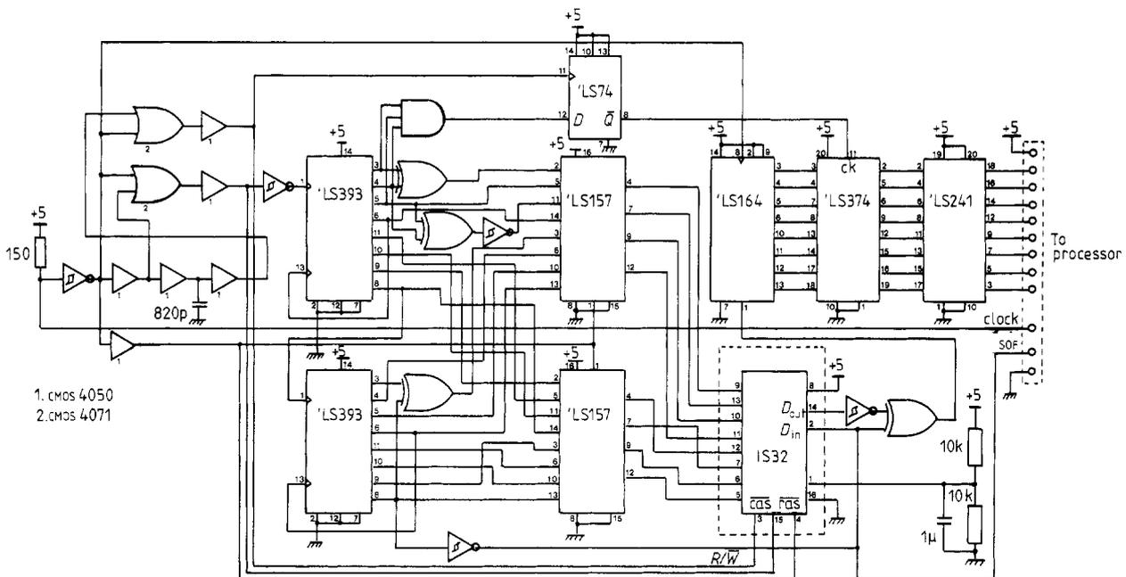
Figure 3. The camera drive electronics.
