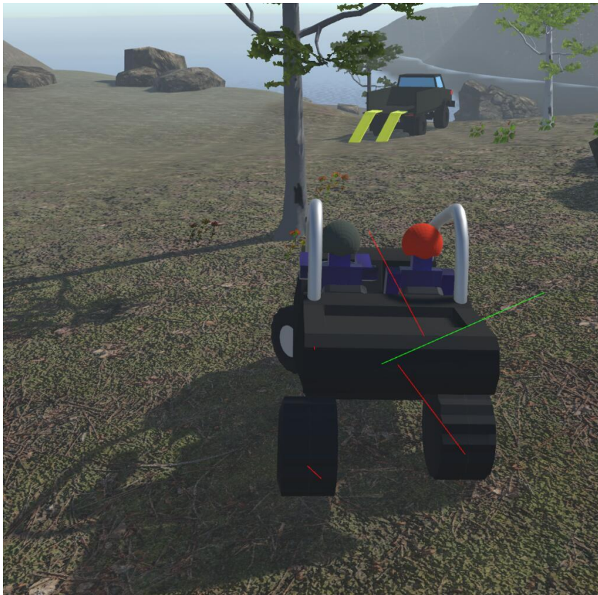
Figure 5: Current force on each wheel is shown in red, and net force on the vehicle in green
