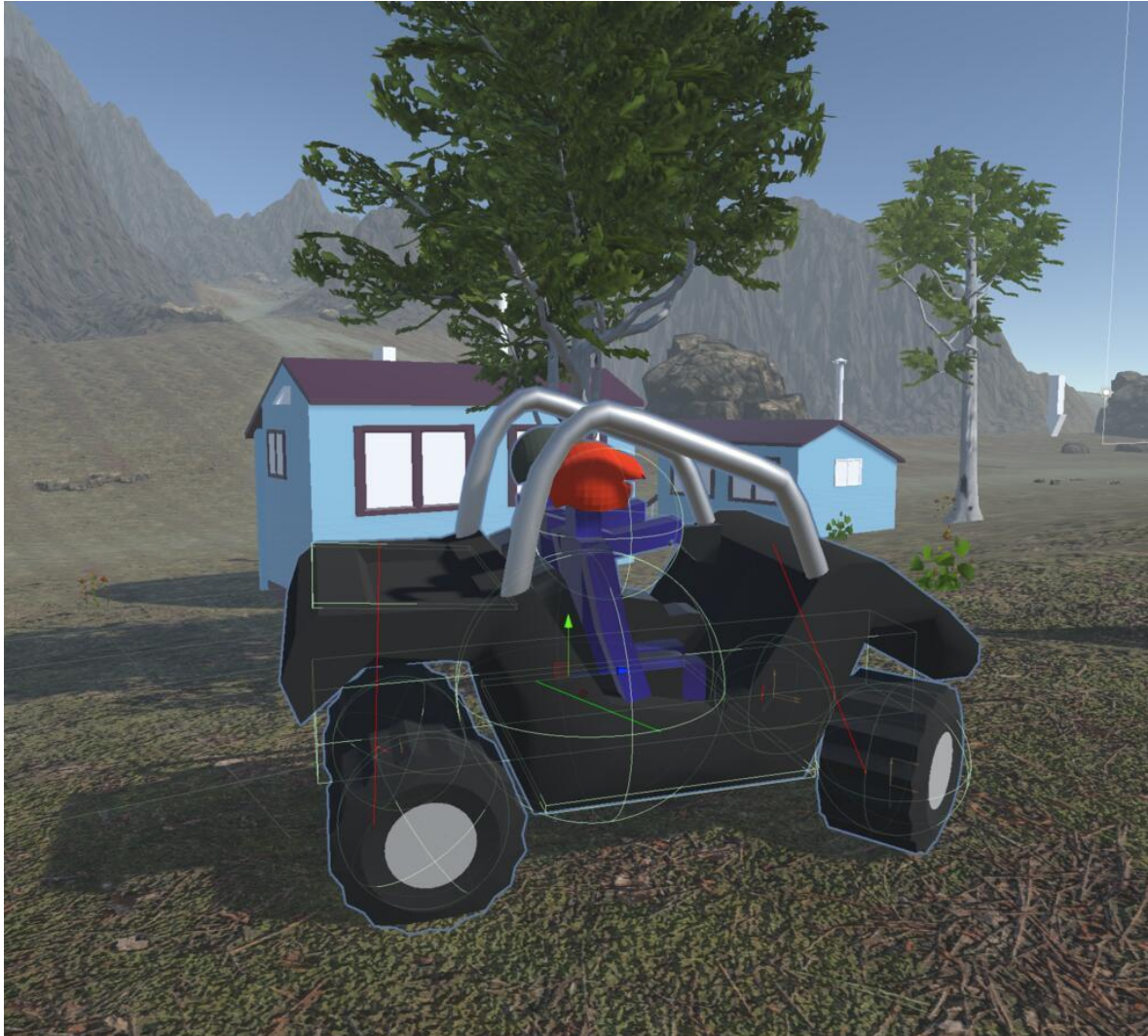
Figure 4: Glowing lines show how each wheel is modelled as a spherical collider on a suspension.
